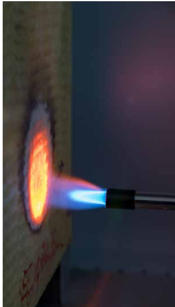
Image 2: Flame impact on the test specimen during the continuous smouldering test
