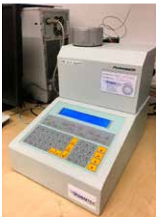
Image 15: Pycnomatic HTC He-pycnometer for determining the solid's volume
