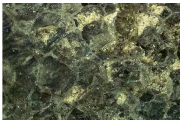
Image 8: Foam glass with superficial structure damage due to frost-thaw cycles
