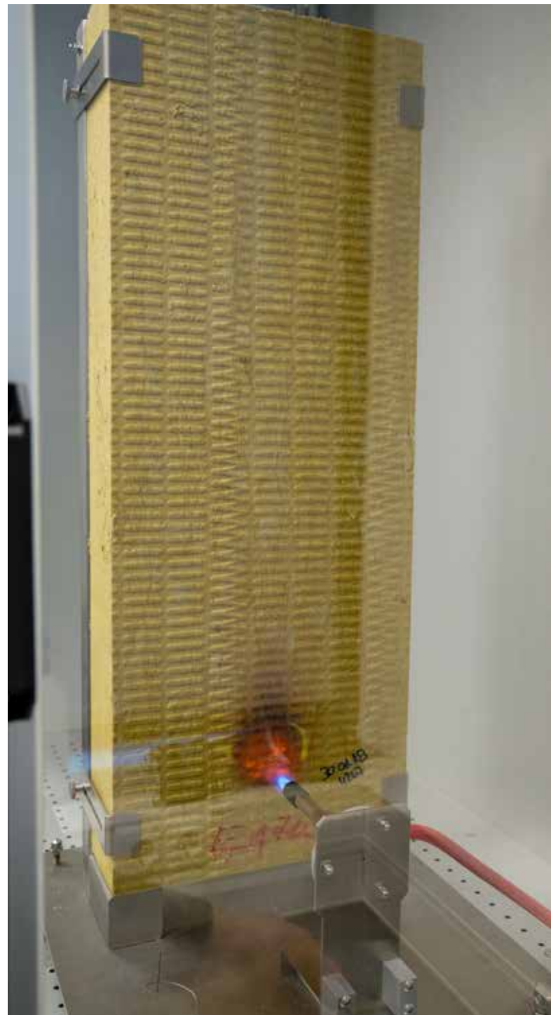
Image 1: Overall view of the testing equipment according to DIN EN 16733 at FIW München
