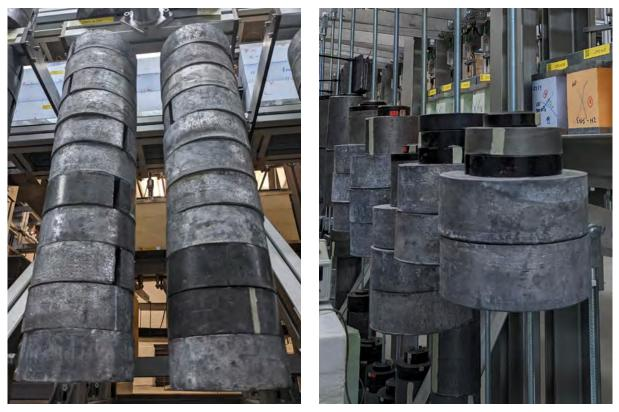
Long-term creep: in some cases large weights on the lever to simulate the substantial load of a building
