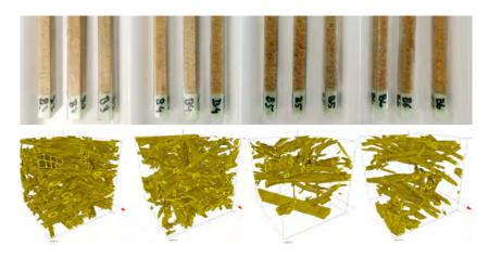
Fig. 1 above: Sample preparation of wood fibre insulation materials of different densities (FIW); below: volume rendering of the variants B3 - B6 based on high-resolution tomographic images (ITWM)
