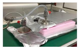
**Fig. 2:** Test specimen for determining the proportions of the heat transfer mechanisms with foil wrapping and flanged evacuation adapter
