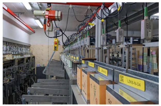
Determining long-term creep behaviour, new test stands with variable sample size
