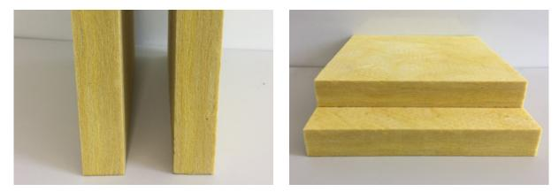
ERM-FC440 (photo left and right): the new reference fibre at FIW München replaces the previous IRMM-440
