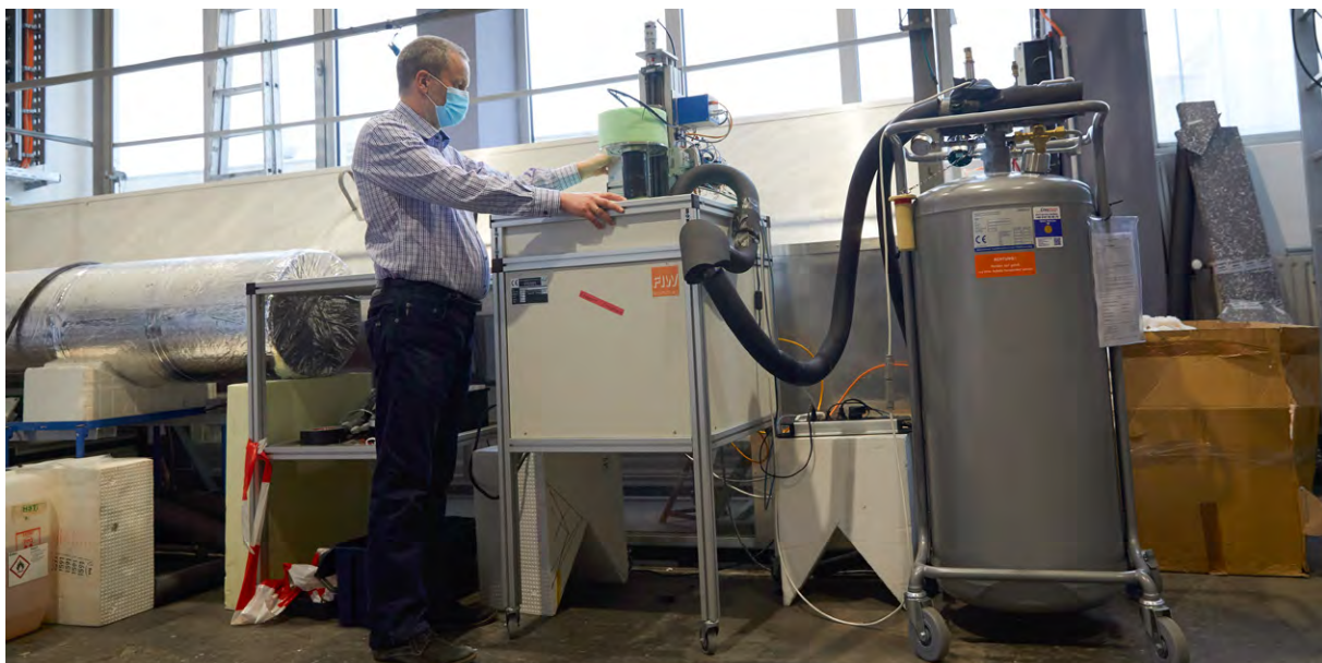
7: Cryogenic laboratory at FIW München, device for determining the linear expansion of cold insulation materials
