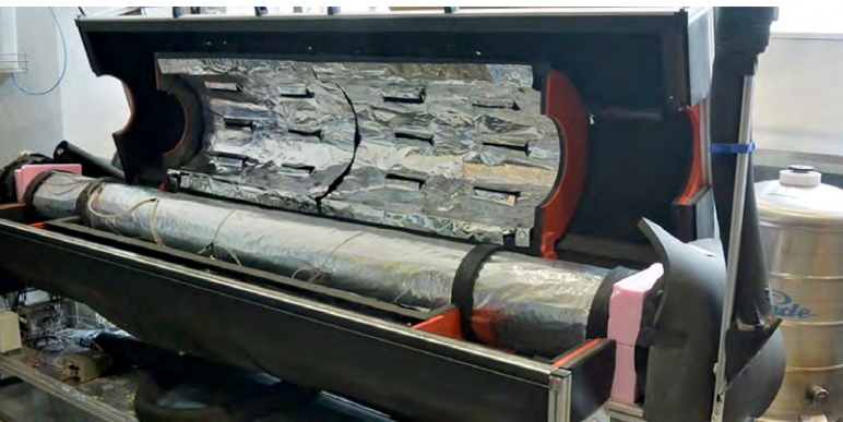
3: Upgrade of the test rig to cryogenic temperatures by using liquid nitrogen
