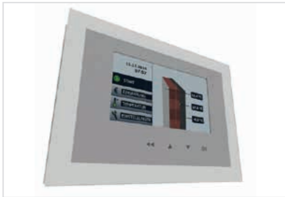
† The pilot production model. The microcomputer with graphical user interface is connected to an insulation plate of exterior insulation that is equipped with sensors. It contains sensors for determining the surface temperature of the outer wall.
