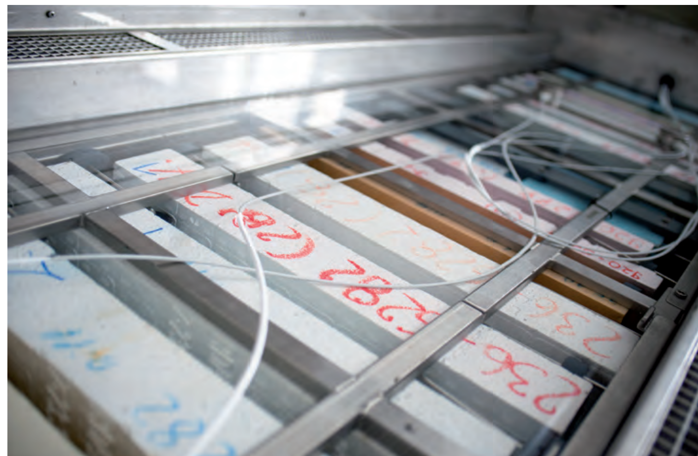
† Testing device to determine behavior during freeze/thaw cycle
