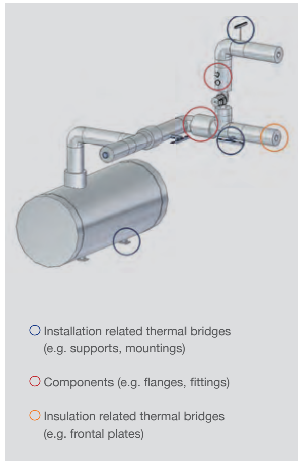
† Holistic approach of a "Technical Insulation" system
