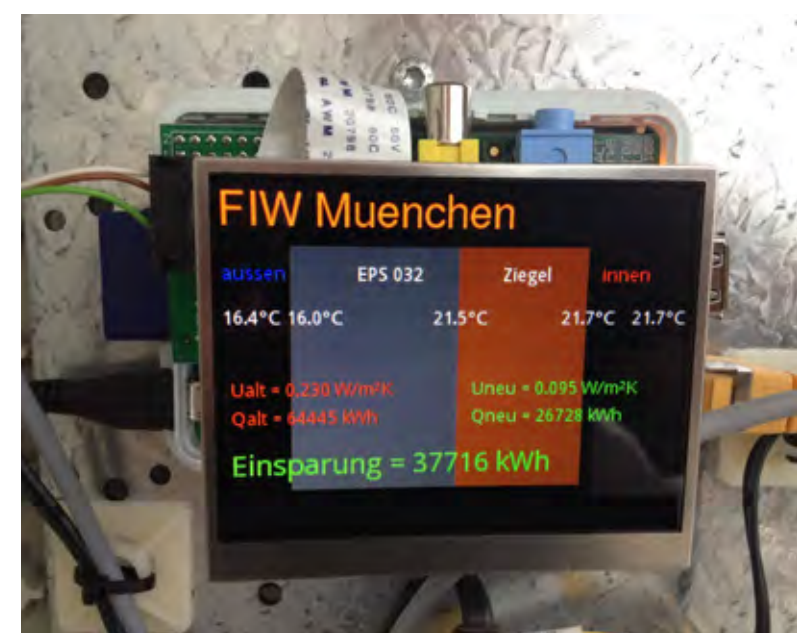
† First prototype of the measuring device
