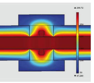
t temperature curve of a FEM-simulation for a bestpractice flange cap
