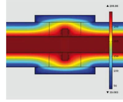
t temperature curve of a FEM-simulation for a flange cap according to the state of technology
