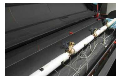
from the beginning to the end of the measurement section. On the other, a heat flow meter is installed whose signal is proportional to the measuring system's heat loss.
