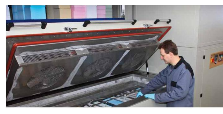
4. Testing equipment to determine water absorption by total immersion
