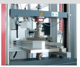
Automation of the compressive test
