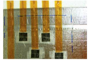
Measurement of thermal conductivity of VIP
