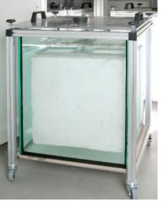
Water absorption of EPS with high thickness
