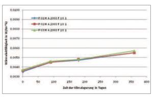
Long-term increase of thermal conductivity for temperature storage of VIPs
