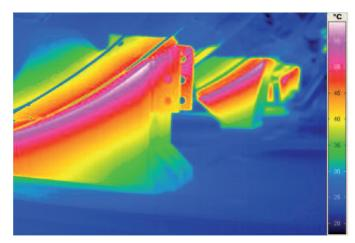
Figure 1: IR image of the uninsulated support of a boiler during operation
