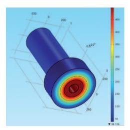
Figure 2: Insulated flange in finite element analysis
